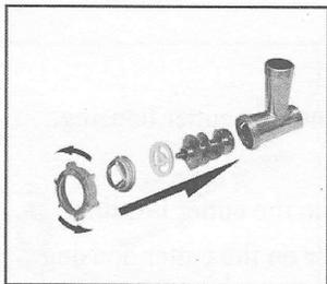
1. Insert the feed screw into the cutter housing, the plastic end first.
