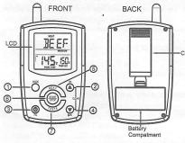
LCD (Liquid Crystal Display) – Displays all icons, temperature and timer. The backlight will flash Blue once the temperature increases 10F, will change to Green when the temperature is within 15F of the set temperature and will turn Red when it reaches the set temperature. See LCD diagram for detailed information.
