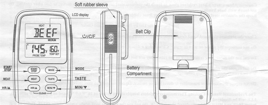
**LCD (Liquid Crystal Display)** – Displays all icons, temperature and timer. The backlight will flash Blue once the temperature increases 10F, will change to Green when the temperature is within 15F of the set temperature and will turn Red when it reaches the set temperature. See LCD diagram for detailed information.
